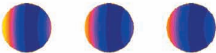
Skin effects visualisation on a set of cables.
