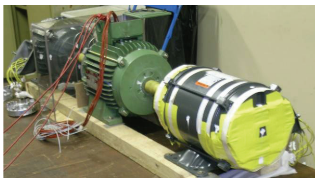
Fig. 4: Test bench with the two motors under test (Motor B in TEFC configuration).
