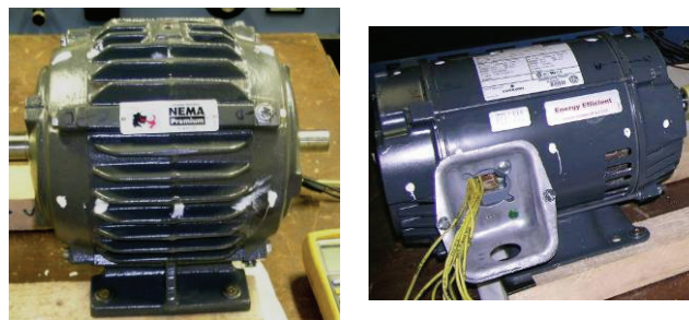
Fig. 3: TEFC Motor A (left) and ODP Motor B (right).
