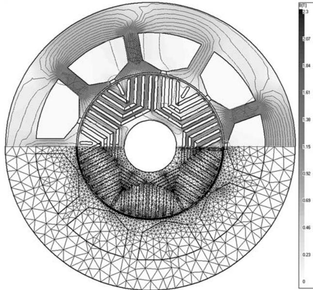
**Fig. 3** FE model of a nine-slots six-pole synchronous reluctance motor design with six-phase concentrated windings
