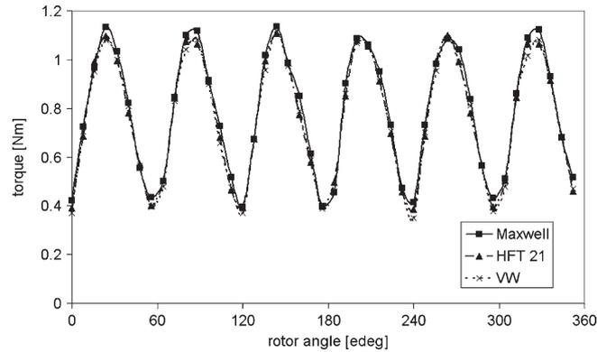
**Fig. 8** Torque estimation for a nine slots six-pole synchronous reluctance motor with three-phase concentrated windings (See Fig. 3)
