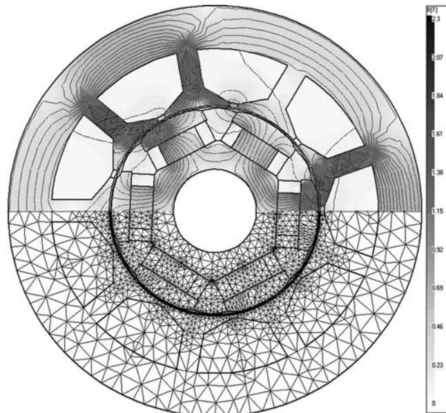
**Fig. 4** FE model of a nine-slots six-pole salient pole wound field motor design with six-phase concentrated windings
