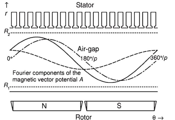
Fig. 1 Explicative for the Maxwell HFT method for computing torque based on the harmonics of the vector potential in the motor air-gap
