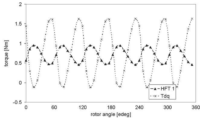
**Fig. 9** Average torque estimation using  $dq$  theory and HFT method for a nine slots six-pole synchronous reluctance motor with three-phase concentrated windings (See Fig. 3)
