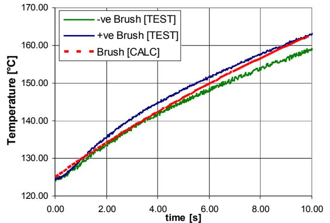
Fig. 10: Measured and calculated brush temperatures for the short Motor 1 (20A for 10 seconds).
