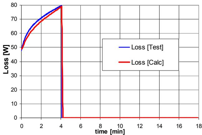
Fig. 17: Measured and calculated total motor loss for Motor 3 with a Powder liner (20A locked rotor until the winding reaches 200C then switched off)
