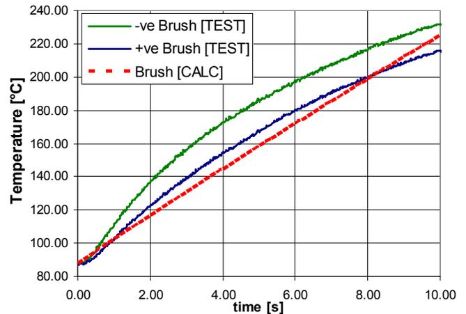
Fig. 11: Measured and calculated brush temperatures for the long Motor 2 (48A for 10 seconds).
