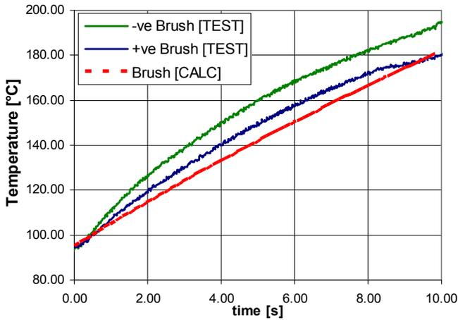
Fig. 12: Measured and calculated brush temperatures for the long Motor 2 (37A for 10 seconds).
