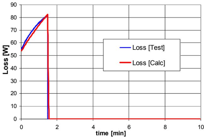
Fig. 16: Measured and calculated total motor loss for Motor 3 with a Nomex liner (20A locked rotor until the winding reaches 200C then switched off)
