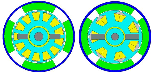
Fig. 1: Radial cross-section for the validation motors (Motors 1 and 2 on the left and Motor 3 on the right)
