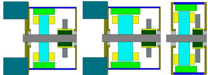
Fig. 2: Axial cross section for the validation motors (Motor 1 on the left, Motor 2 in the centre and Motor 3 on the right)
