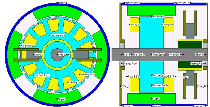
Fig. 7: Motor 2 radial and axial cross-sections showing the positions of nodes in the model (brush holders whose thermal capacitance are included in the model are also shown).
