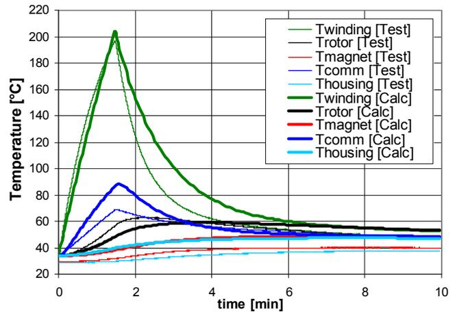
Fig. 14: Measured and calculated temperatures for Motor 3 with a Nomex liner (20A locked rotor until the winding reaches 200C then switched off)
