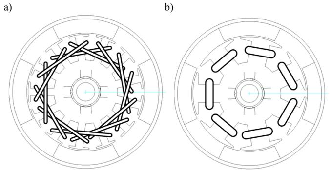
Fig. 6: Armature winding of calculated motors: a) Motors 1 and 2 (simplex wave winding); b) Motor 3 (single tooth winding)
