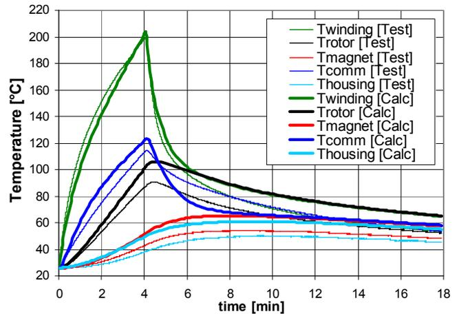
Fig. 15: Measured and calculated temperatures for Motor 3 with a Powder liner (20A locked rotor until the winding reaches 200C then switched off)
