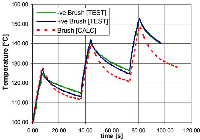
Fig. 13: Measured and calculated brush temperatures for the short Motor 1 (duty cycle of 20A for 7.5 seconds followed by 30 seconds off).
