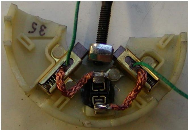
Fig. 4: Motor 1 brush card with thermocouples attached
