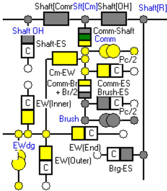
Fig. 9: Thermal network for the commutator and brushes
