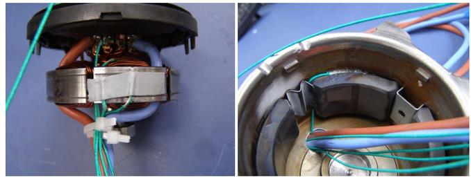
Fig. 5: Motor 3 rotor and stator with thermocouples attached
