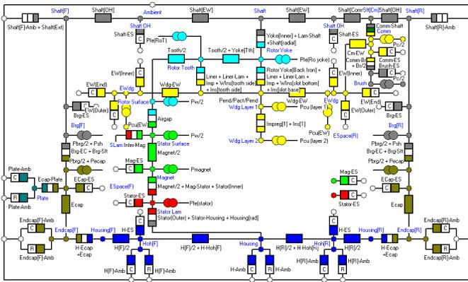
Fig. 8: Thermal network for the PMDC motor
