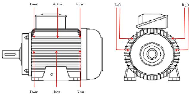
Fig. 3: Temperature measurement points.
