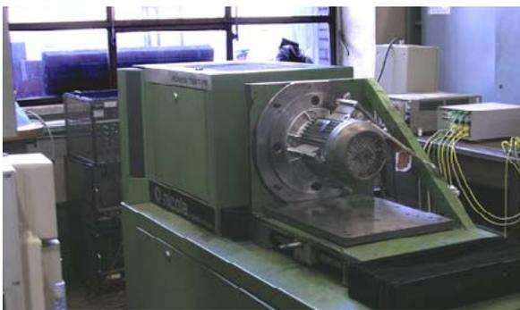
Fig.4: Test bench for the AC load test.
