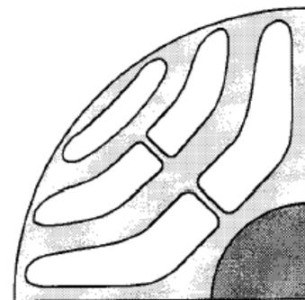
Fig. 1: Schematic of rotor lamination of a Transverse Laminated Synchronous Reluctance Motor (SynRM).
