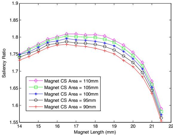
Figure 5-Variation of Saliency Ratio with Magnet Length
