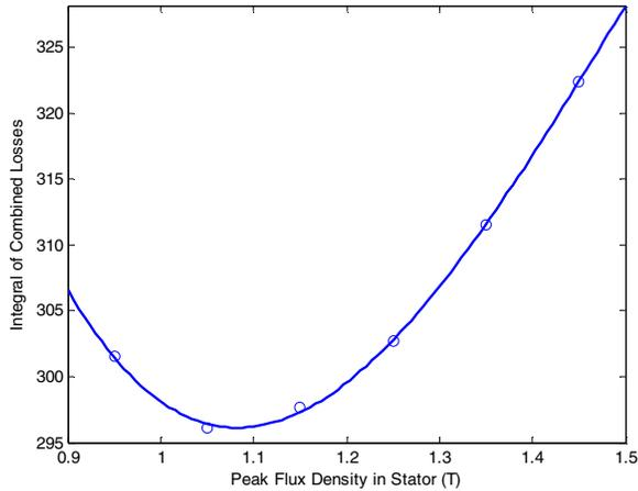
Figure 11-Integral of Combined Losses across the Rated Torque and Power Characteristic against Stator Flux Density
