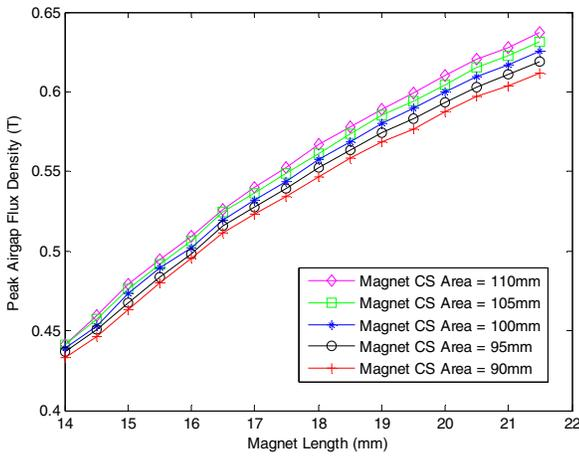
Figure 4 -Variation of Airgap Flux Density with Magnet Length
