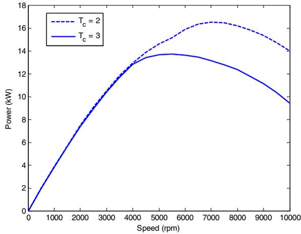
Figure 15- Thermally Constrained Continuous Maximum Power Envelope
