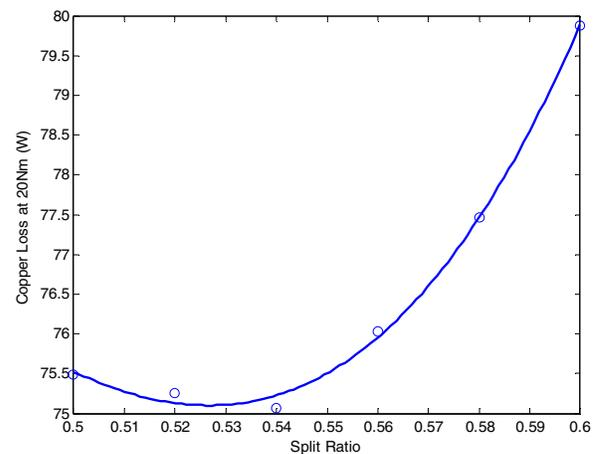
Figure 2- Variation of Copper Loss at 20Nm with Split Ratio
