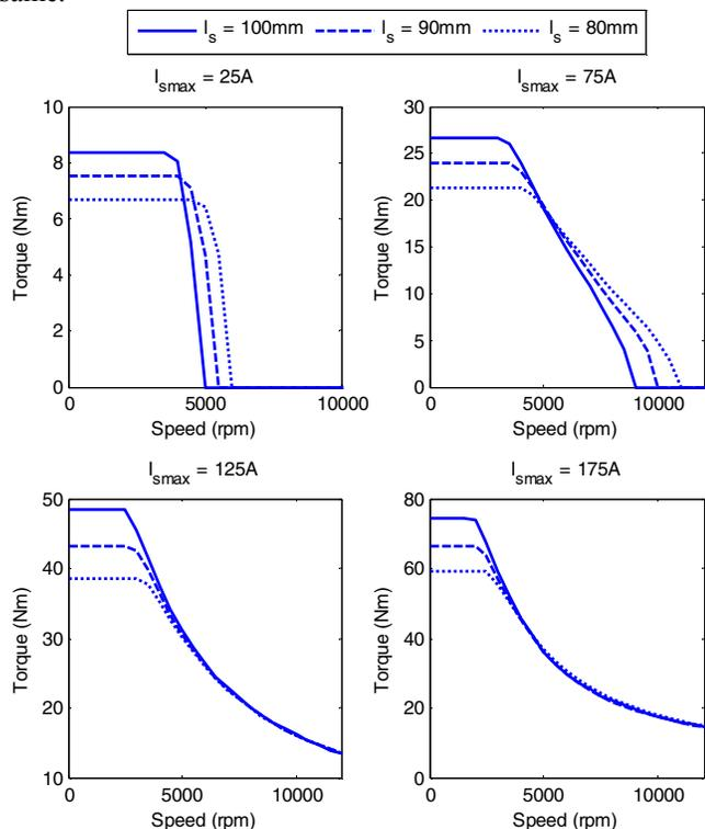
Figure 13-Influence of Active Length on Torque/Speed Characteristics
