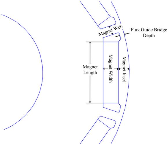
Figure 3-Magnet and Flux Guide Dimensions
