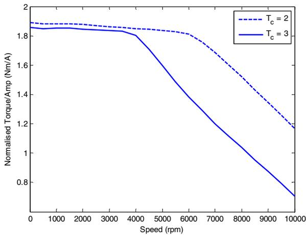
Figure 16-Normalised Torque/Amp for the Continuous Torque Envelope
