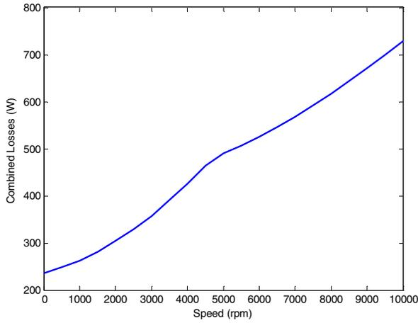
Figure 10-Combined Losses across the Rated Characteristic
