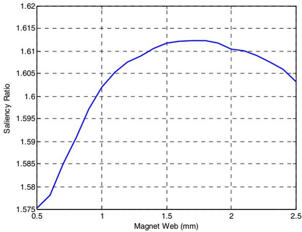
Figure 7-Variation of Saliency Ratio with Magnet Web
