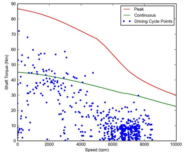
Figure 18- Peak and Continuous Thermal Envelope with Drive Cycle Points
