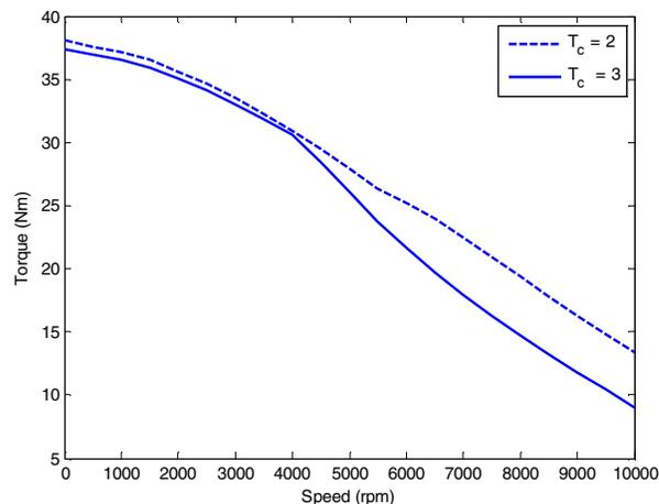
Figure 14-Thermally Constrained Continuous Maximum Torque Envelope
