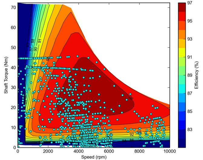
Figure 12-An Efficiency Map with Driving Cycle Points
