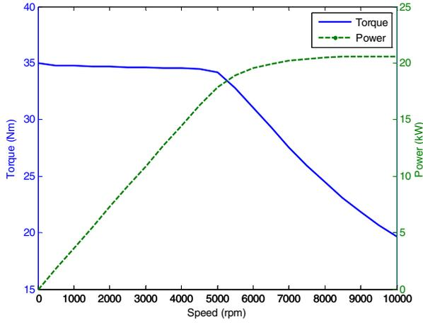
Figure 9-Rated Torque and Power Characteristic
