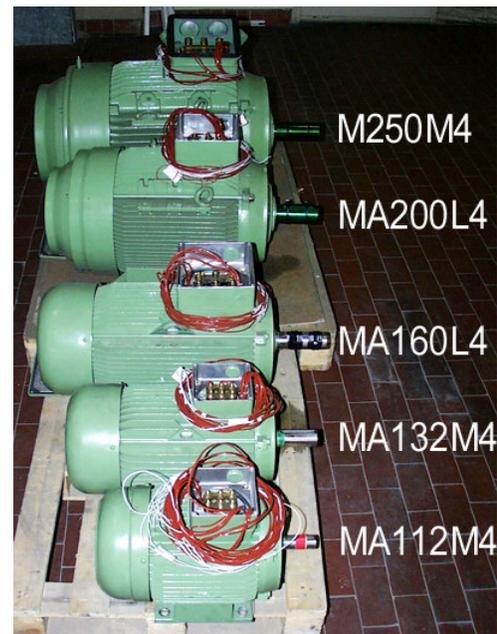
Fig. 1: TEFC motors used to generate test data.
