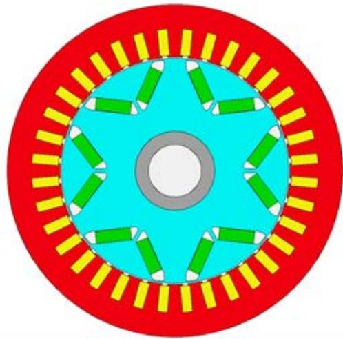
Fig. 7 - The Motor-CAD model of the 36-slot/6-pole machine.
