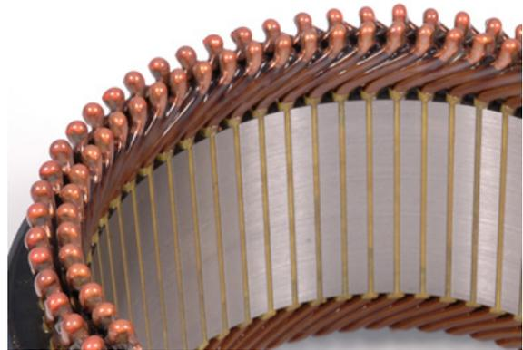
Fig. 1 - Example of a hairpin winding (Source Remy)
