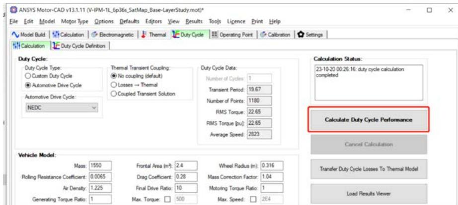
Fig. 15 - Drive cycle analysis in Motor-CAD.
