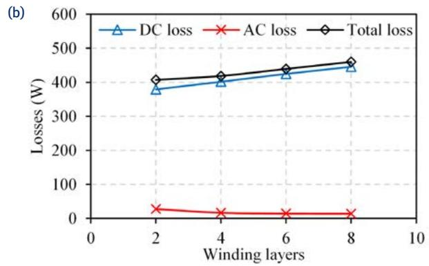
Fig. 14 - Winding losses of the machines with different winding layers. (a) At 12,000rpm, 200A. (b) At 1,000rpm, 200A.
