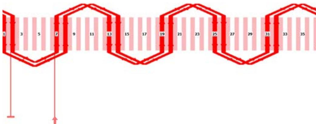
Fig. 11 - Linear view of the winding of phase 1 in Motor-CAD.
