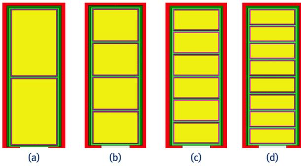
Fig. 12 - Slot view of machines with different winding layers. (a) 2 layers. (b) 4 layers. (c) 6 layers. (d) 8 layers.
