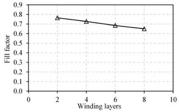
Fig. 13 - Slot fill factors with machines with different winding layers.
