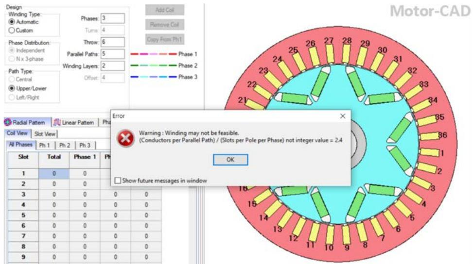
Fig. 6 - Hairpin design check in Motor-CAD showing warning message as design is not feasible.
