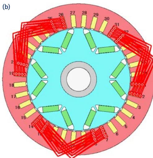
Fig. 10 - Hairpin winding definition in Motor-CAD. (a) Winding definition and coil patterns. (b) Coil arrangement of phase 1 in Motor-CAD.
