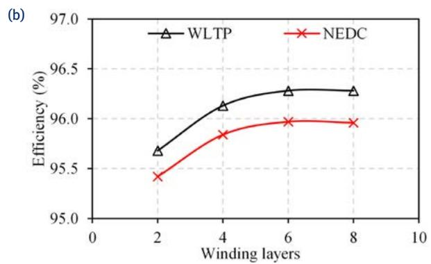
Fig. 16 - Copper loss and efficiency for different drive cycles. (a) Copper loss. (b) Efficiency.
