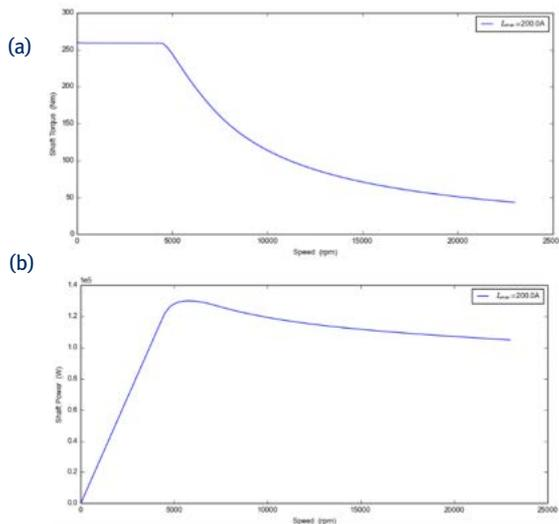
Fig. 8 - Motor performance curves. (a) Peak torque vs. speed. (b) Peak power vs. speed.
