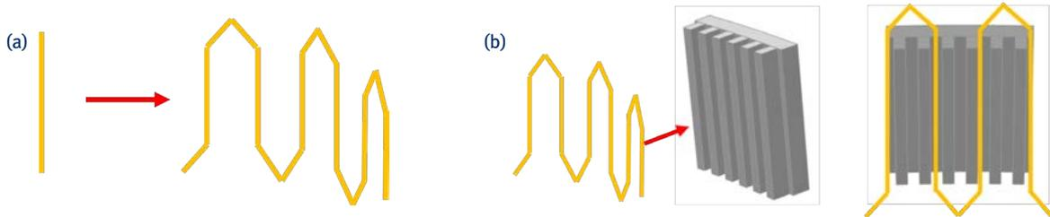
Fig. 4 (a-b) - The production process of the winding with radial-insert hairpin conductors. (a) Shaping of the wire. (b) Assembling the pre-formed winding to the motor.
