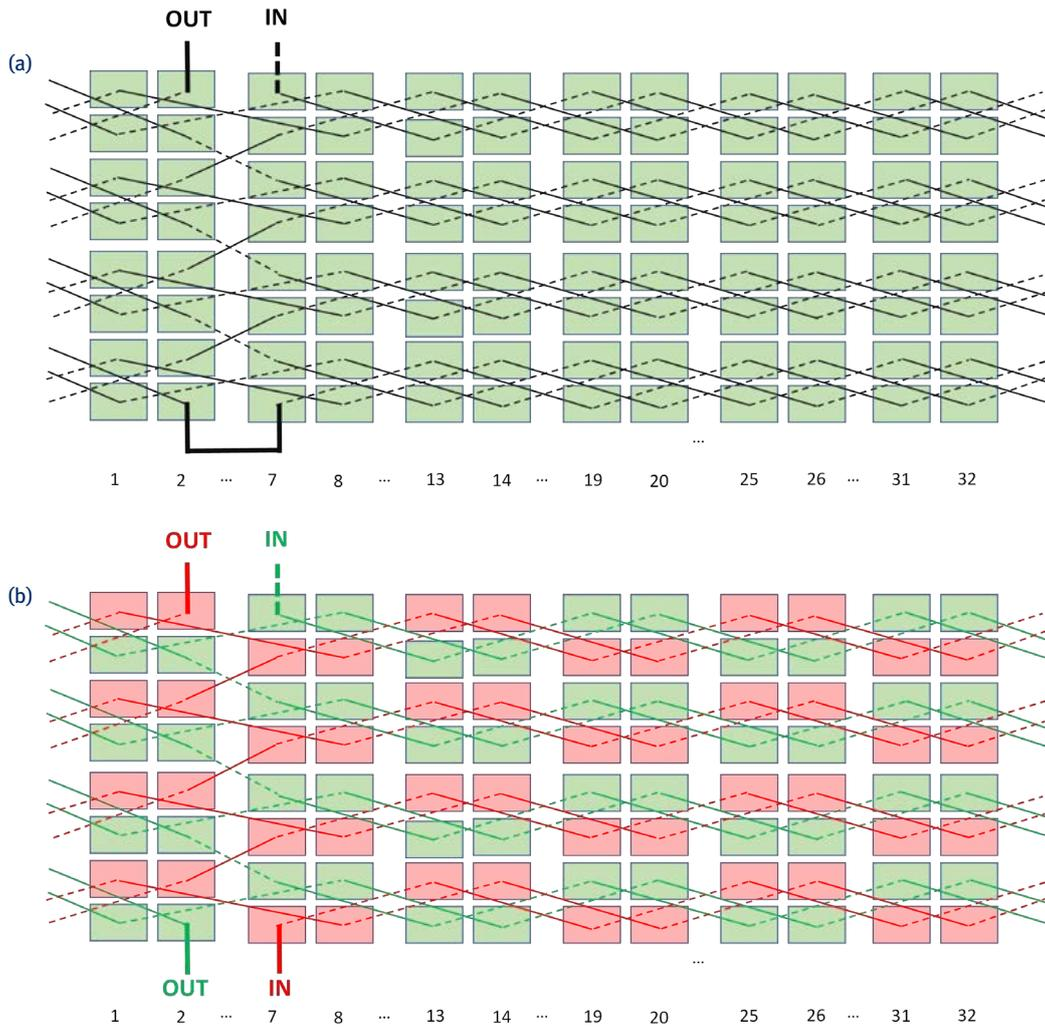
Fig. 5 - Hairpin winding configurations with different number of parallel paths. (a) 1 parallel path. (b) 2 parallel paths.
